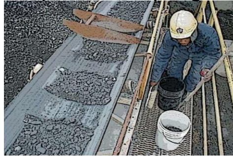
FIGURE 6. Automatic mid-belt samplers are used with belt conveyors
